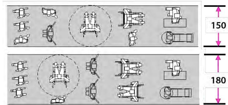
Figure 5. Required dimensions for paths for manual wheelchairs (in cm)
