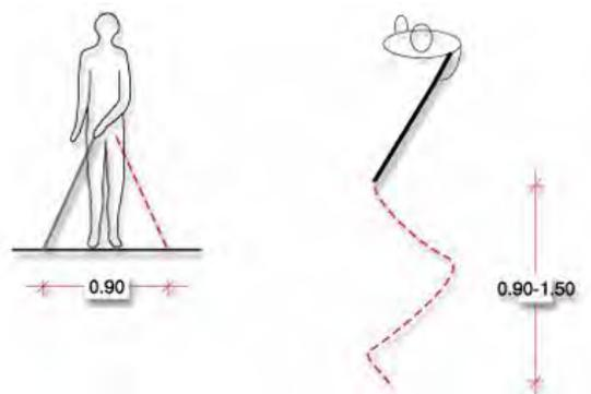
Figure 10. Detection zone for white canes (in m)
