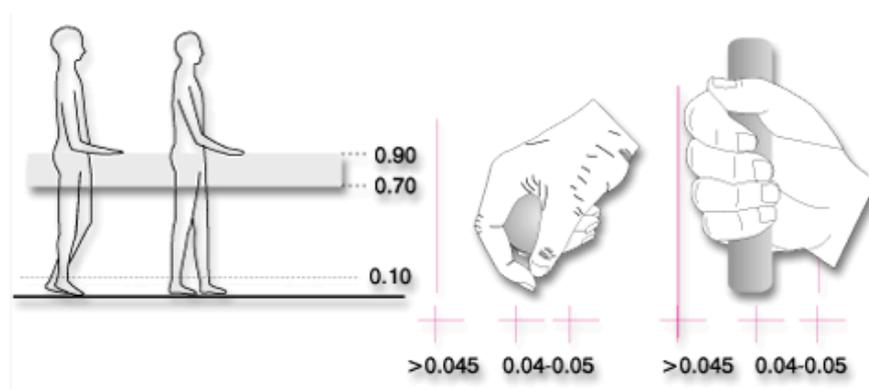
Figure 9. Zones for vertical installation of handrails and handles (in m)
