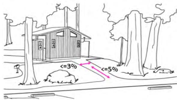
Figure 17. Minimum path slopes (in m)
