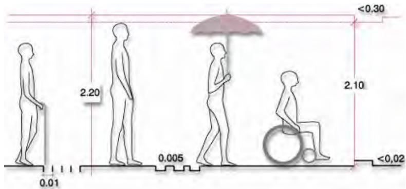
Figure 18. Free passage height and tolerable surface distortions
