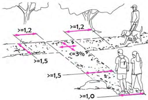
Figure 16. Minimum path widths (in m)
