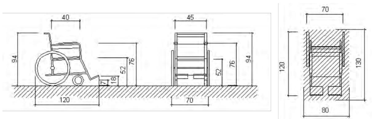
Figure 1. Dimensions of manual wheelchair in cm (side view on the left, rear view in the middle and top view on the right)
