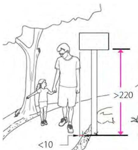
Figure 34. Directional sign placement (measurements in m)
