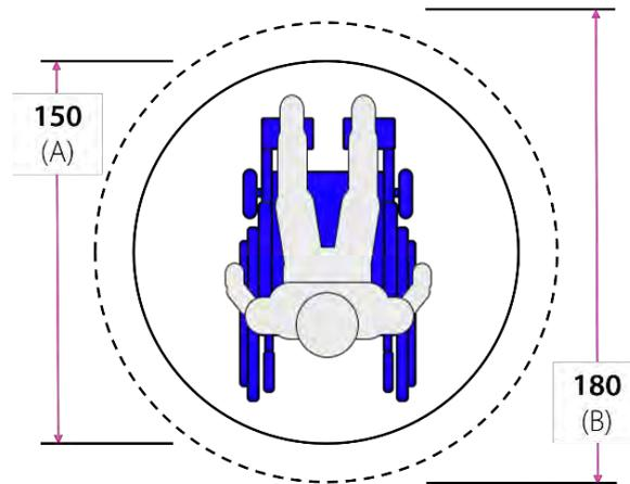
Figure 3. Required dimensions for turning a manual wheelchair (in cm)
