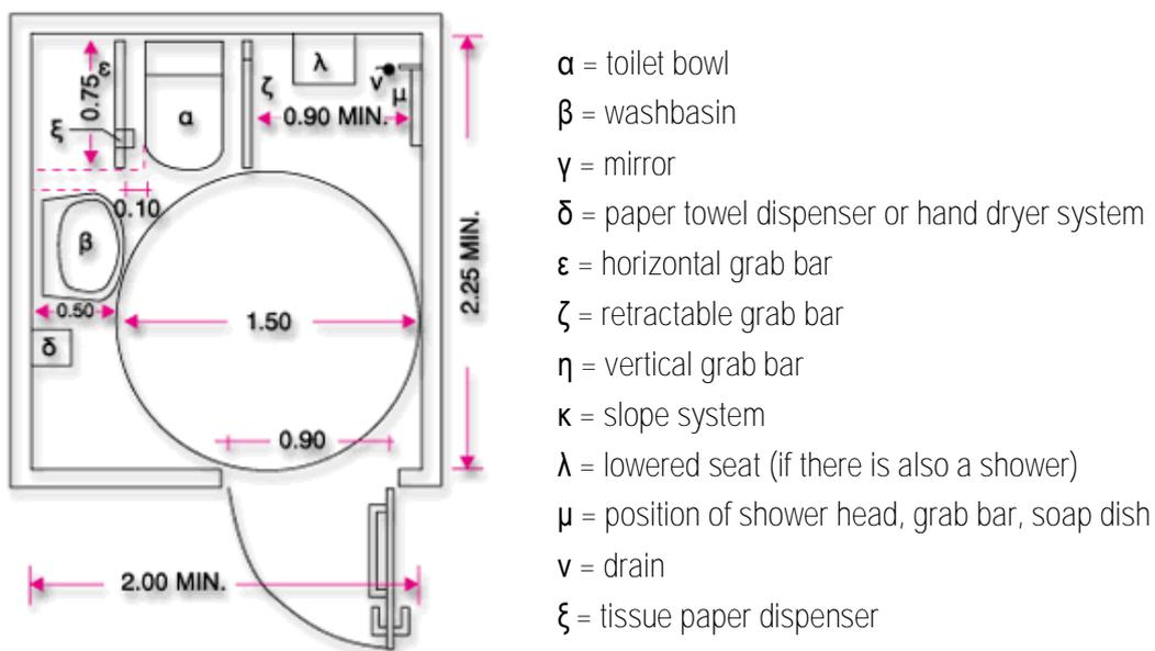
Figure 30. Restroom with turning space and washbasin inside the cubicle (measurements in cm)
