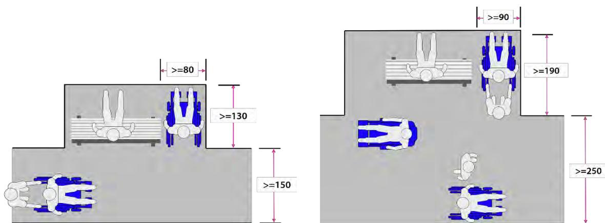
Figure 20. Minimum (left) and ideal (right) dimensions for rest areas as an extension to the paths
