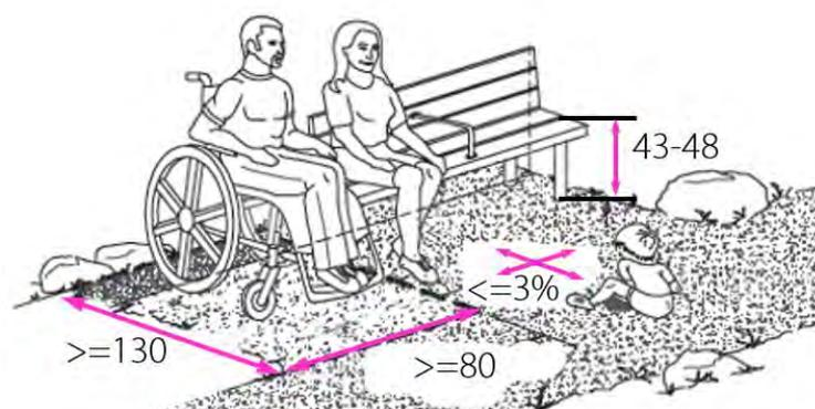
Figure 21. Minimum slopes and dimensions for rest areas as an extension to the paths
