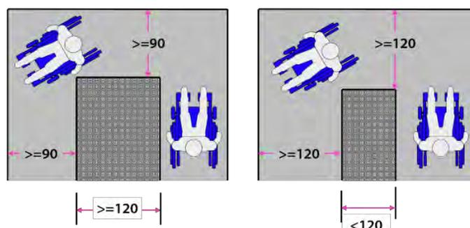
Figure 22. Minimum required dimensions for a wheelchair user to manoeuvre around an obstacle
