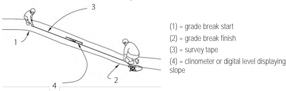
Figure 50. Calculating a slope using a clinometer or a digital level
