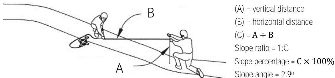
Figure 48. Calculating slopes using measuring tapes/rods
