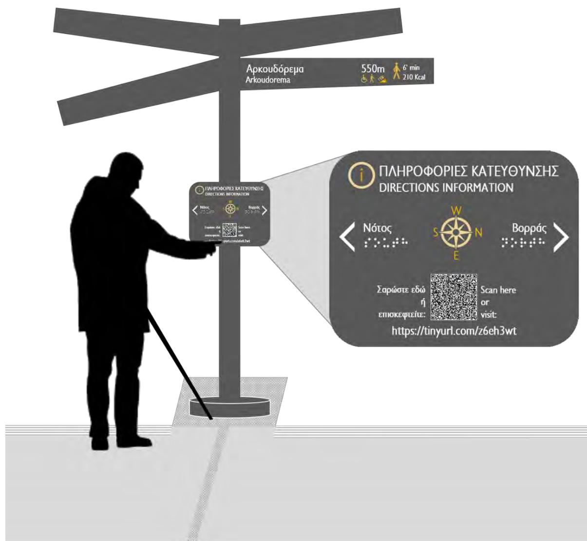
Figure 35. Example of accessible directional signage with tactile sign and additional provisions for the blind<sup>12</sup>
