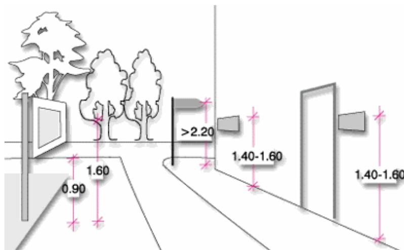
Figure 31. Sign position (measurements in m)
