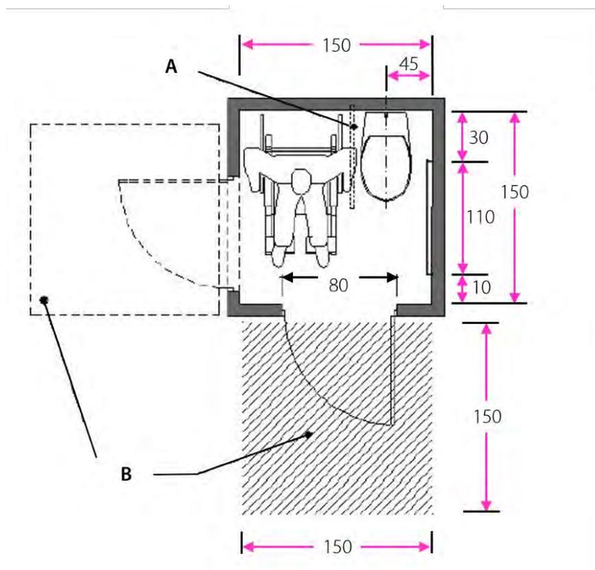
Figure 29. Restroom with turning space and washbasin outside the cubicle (measurements in cm)
