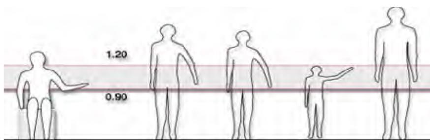
Figure 8. Zones for vertical installation of control mechanisms (in m)
